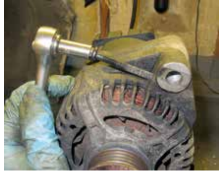
This 8mm bolt on the alternator adjusts the tension on the drivebelt, but is often seized and will snap if turned.
